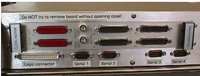
Figure 3: Housekeeping crate rear connectors
