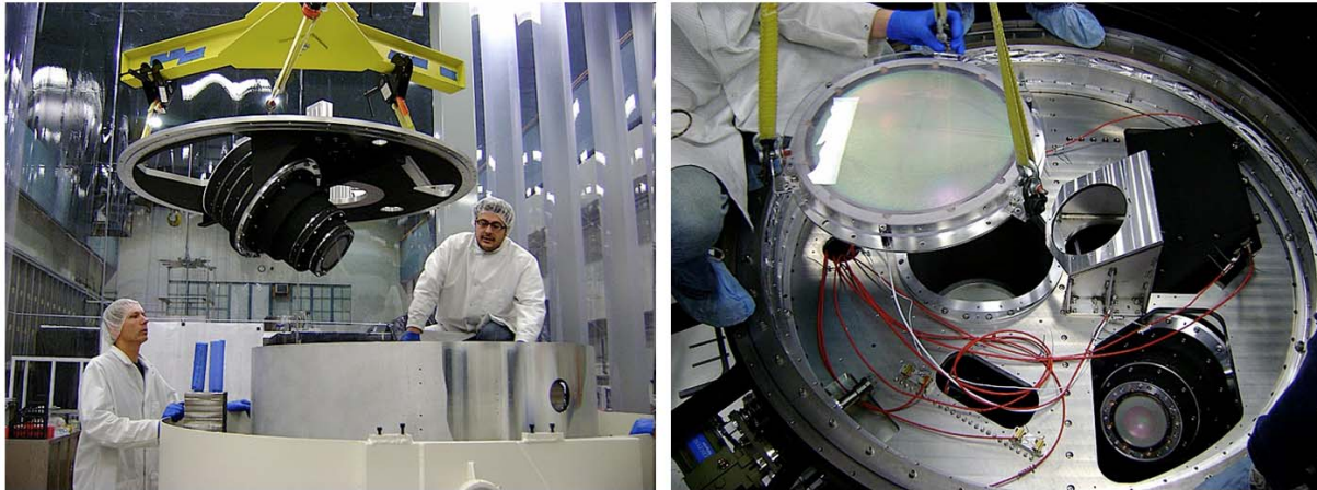
Figure 5: Left, installation of the completed camera barrel. Right, installation of the large CaF 2 field lens.
