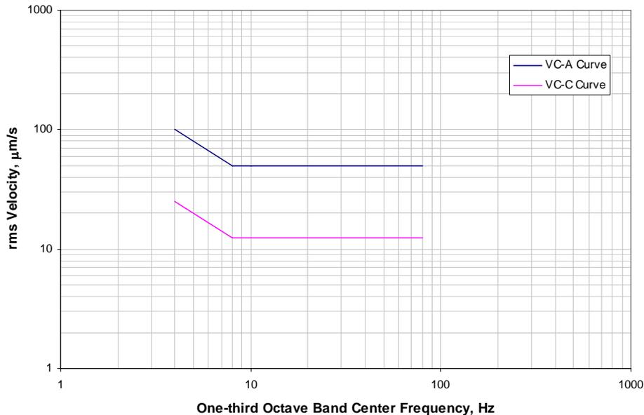
**Figure 3: Keck I Telescope Equipment Vibration Limits**
