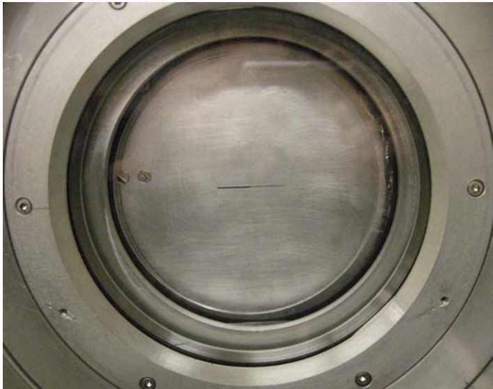
Figure 2. FLITECAM's entrance slit. The left side of the slit is 2" wide, while the right side is 1" wide.
