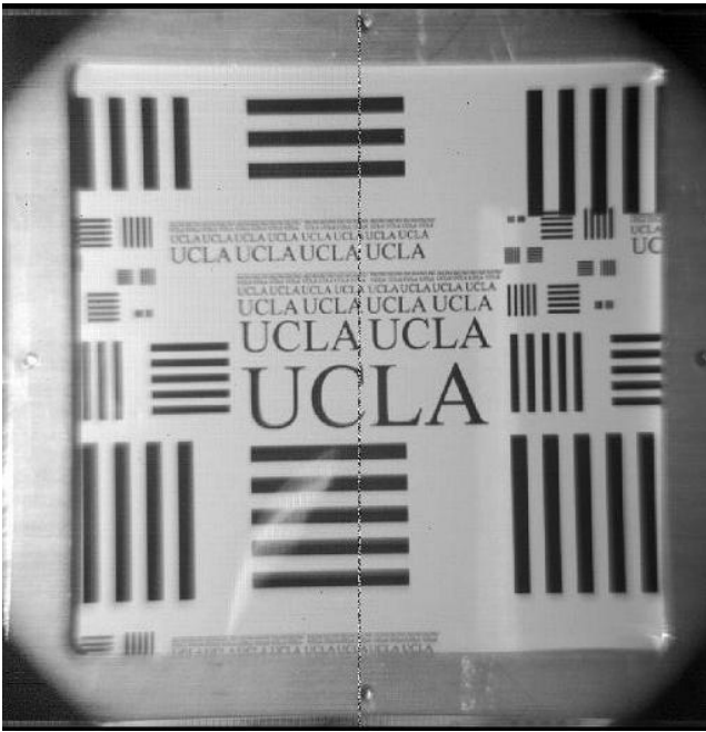
Figure 6: A test pattern imaged with FLITECAM using a bare ALADDIN multiplexer at room temperature.
